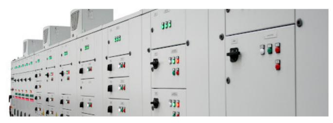
A Motor Control Center (MCC) is an assembly of one or more enclosed feeder sections having a common power bus bar and principally containing Motor Control units. Motor Control Centers are having several Motor Starters assembled in one common panel. A Motor Control Center can also include Variable Frequency Drives (VFD), Programmable Logic Controllers (PLC).
